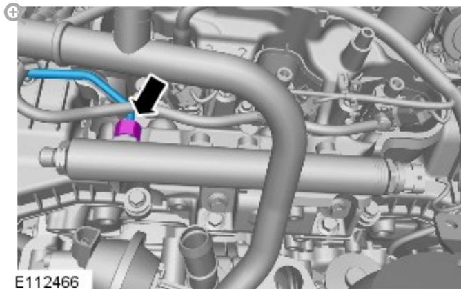
Tighten the high-pressure fuel lines union to 15Nm.
