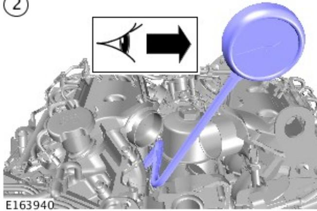
Crank the engine for 10 seconds and record the figure displayed on the compression test gauge. Make sure the pressure is released from the compression test gauge after each cylinder recording. Repeat the process for all cylinders.
