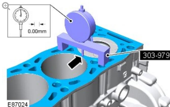
Zero the gauge on the cylinder block machined face.
