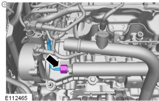
Tighten the high-pressure fuel line union to 30Nm.
