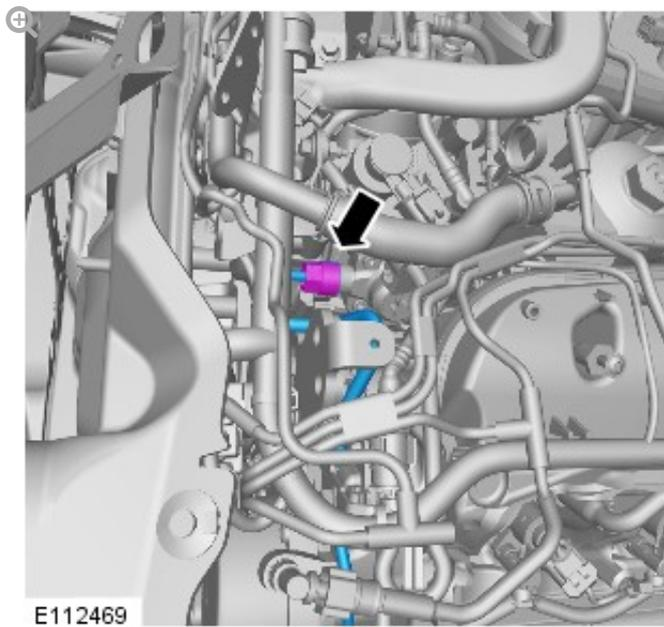
Tighten the high-pressure fuel lines union to 15Nm.
