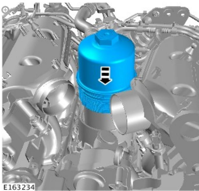
Install the oil filter element and housing.
