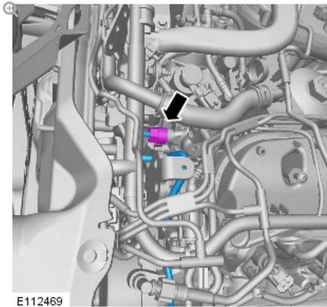
Tighten the high-pressure fuel line union to 30Nm.
