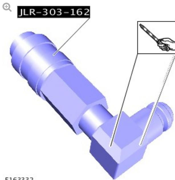
Using a suitable tool, remove the corner edges of special tool JLR-303-1629 as illustrated.
