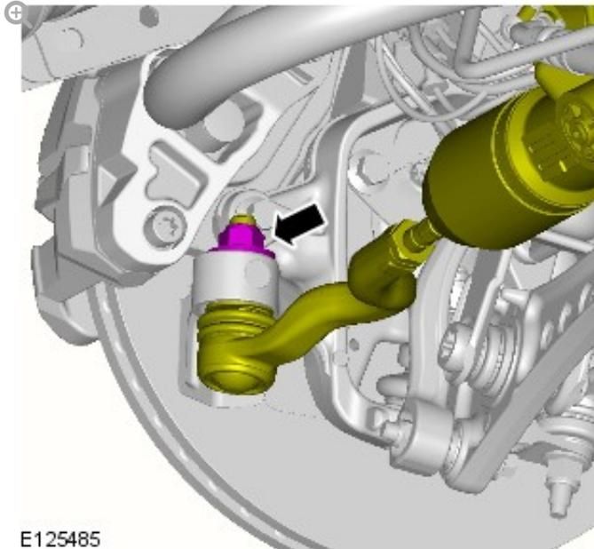
Remove and discard the nut. Install a new nut.
