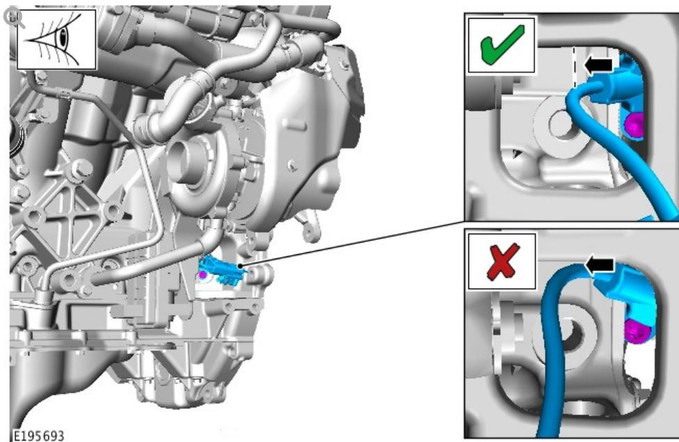
Using the illustration, check the installed position of the CKP sensor as seen through the cylinder block opening. The CKP sensor wiring must point towards the 9 o'clock position and not contact the cylinder block as shown. If the position is not correct repeat the process from step 10 of the removal procedure.
