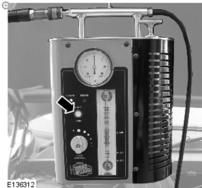
Switch the smoke test equipment on.
