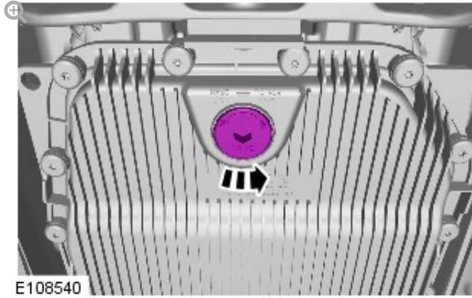
Discard the transmission fluid drain plug.
