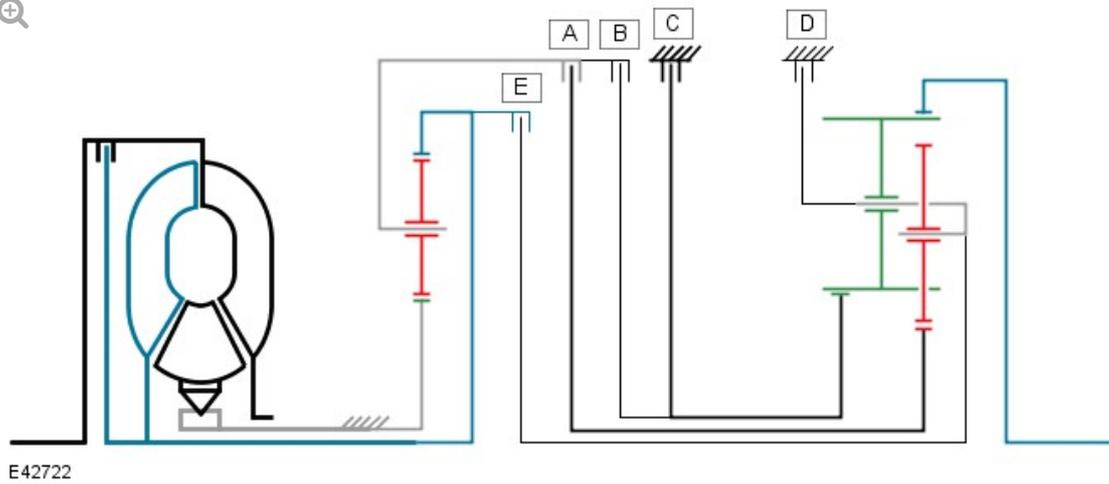
The JaguarDrive selector and the selector spool valve are in the 'D' position. Engine torque is transmitted from the torque converter turbine shaft to the ring gear 1 of the single web planetary gear train and the outer plate carrier of clutch 'E'.
