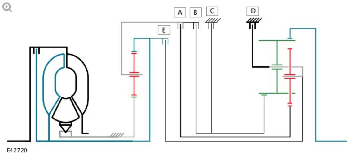
The JaguarDrive selector and the selector valve spool are in the 'D' position. Engine torque is transmitted from the torque converter turbine shaft to the ring gear 1 of the single web planetary gear train and the outer plate carrier of clutch 'E'.
