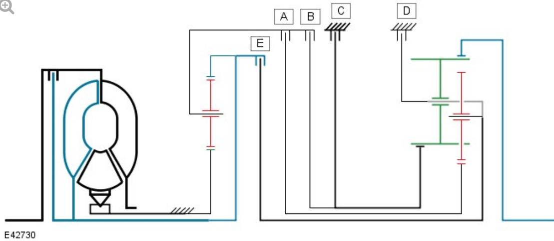
The JaguarDrive selector and the selector spool valve are in the 'D' position. Engine torque is transmitted from the torque converter turbine shaft to ring gear 1 of the single web planetary gear train and the outer plate carrier of clutch 'E'.
