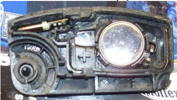
Open upper and lower portion of key Fob. See the Transponder chip in the upper right corner. The Transponder chip is incased in a silicone tube but that tube was removed for illustrative purposes.
