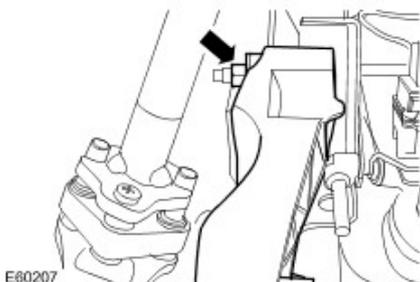
6 . Manual vehicles only: Remove the pedal from the clutch master cylinder.
